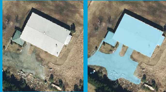
Impervious area is shaded in blue on this aerial image of a property.
